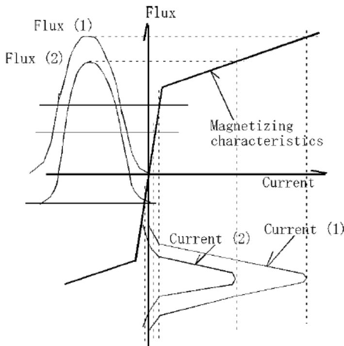
Fig. 1.6 Magnetizing current under d.c. current superimposed
