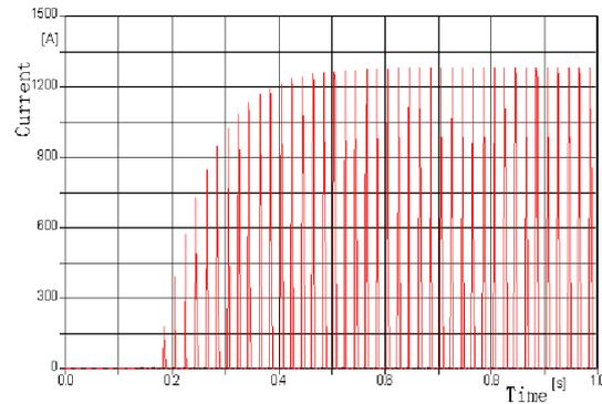
Fig. 1.8 ATP-EMTP calculation of transformer magnetizing current under geomagnetic storm
