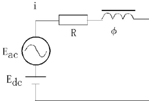
Fig. 1.7 Circuit diagram for geomagnetic storm condition
