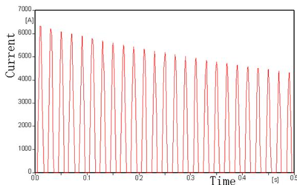
Fig. 1.5 Transformer magnetizing current
