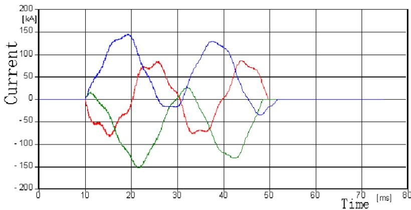
Fig. 1.3 Short-circuit currents in EHV sub-station
