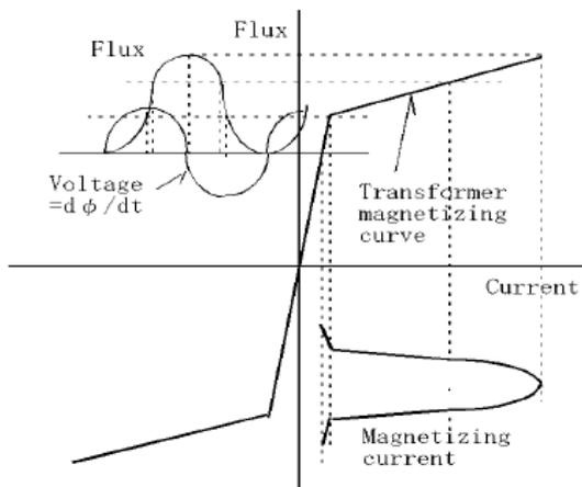
Fig. 1.4 Transformer inrush magnetizing current
