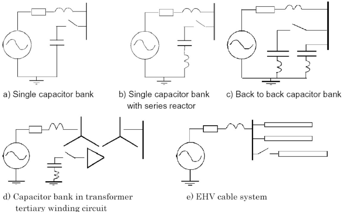
Fig. 1.9 Circuit diagrams creating capacitive inrush currents
